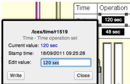
Clicking writeable node value opens write dialog box. The current edit node marks with four black squares. There are two kinds of write dialog window - one for numerical value and one for On/Off set value. The upper part displays the online current node state. The lower part is used to modify the node state value.
