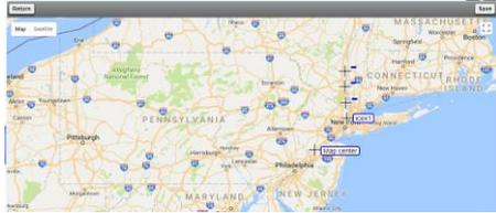
Locate screen allow dragging the units to their exact location, to drag the map center to the right position and to set the suitable map resolution.
