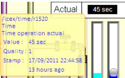
Positioning the mouse over writeable graphical elements will change the mouse cursor to a hand cursor. A hand cursor indicates that clicking the element will perform an action, such as set, reset and toggle an element, switching to a screen, or opening a edit dialog window.
